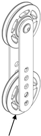
Adjust the tension of the Cable System by moving the lower Pulley position on the Double Floating Pulley Brackets.
