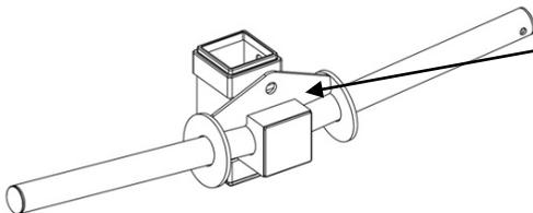
**Ensure the triangular cable connection bracket on Sliding Weight Post faces up and back.**
